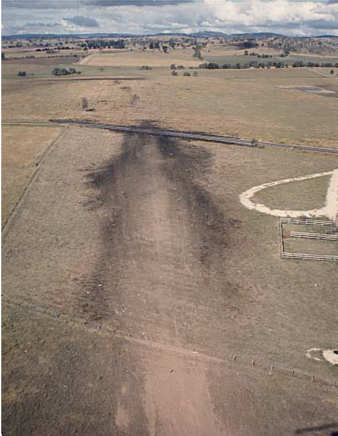
Ground impact scar – aircraft A8-128
