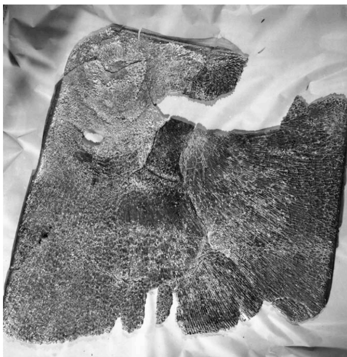
Birdstrike damage to pilot's side canopy – aircraft A8-133
